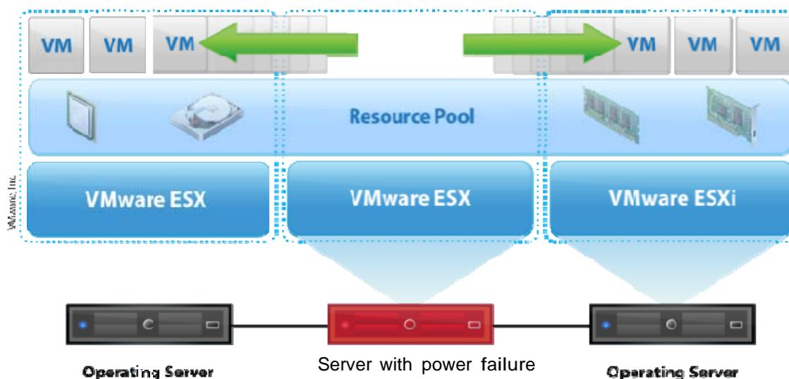
**Figure 2.** Sophisticated power management solutions maintain business continuity during power failures by automatically migrating virtual machines to unaffected parts of the network or to an offsite backup facility, colocation data centre or cloud computing infrastructure.<sup>1</sup>
