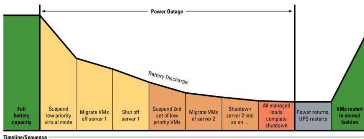
**Figure 3.** Should a power outage threaten to outlast UPS battery capacity, advanced power protection software can shut down impacted servers automatically and gracefully.
