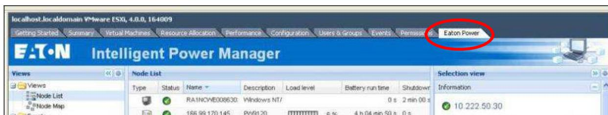
**Figure 1.** Plug-ins now available with some power management solutions integrate closely with leading virtualisation management systems, enabling technicians to view, monitor and administer all of their server, storage and power management assets through a single console.
